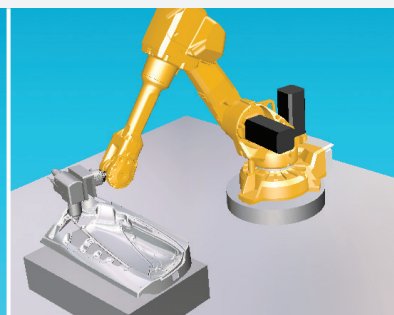
Laser Cut and Material Addition
