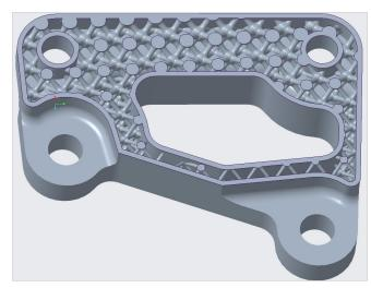
Create lattices with parabolic beams.
