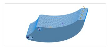
The Topology Optimization basic workflow includes: define regions, loads and constraints, mesh the part, then run the optimization
