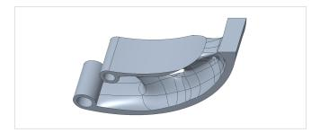
The standard output of the Topology Optimization can be converted to a solid model in the form of a Creo freestyle feature. STL format is another option.
