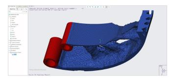
The standard faceted output of the Topology Optimization can be displayed at the end of the process or at any time during the run cycle.
