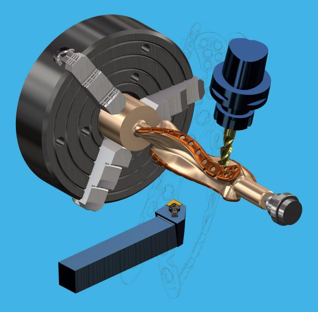
Automate your complex programs for high-powered, multitasking machining centers. Program it right the first time, every time.
